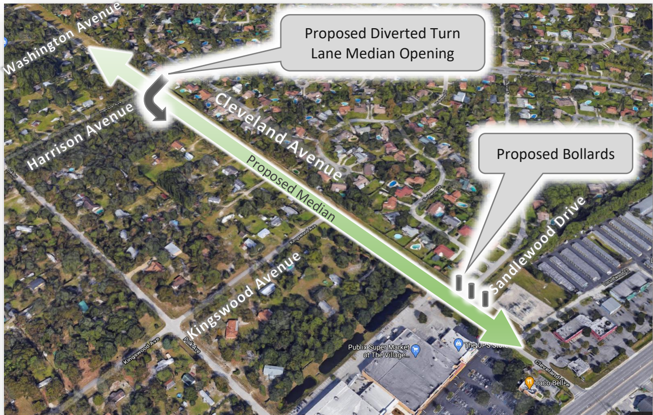
Figure 40: Proposed Cleveland Avenue Median Location and Access Management (Diverted Turn Lane and Bollards)
