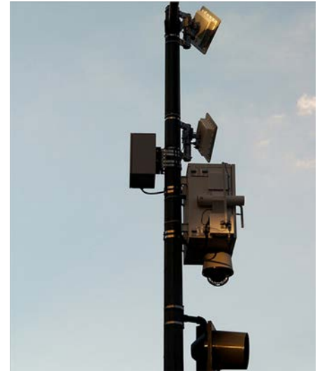
ShotSpotter sensor with pan-tilt-zoom surveillance camera at an intersection in Washington, DC.
