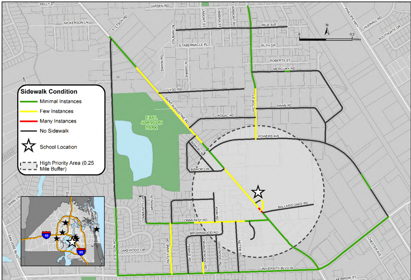
FIGURE 3-43 SAN JOSE SIDEWALK CONDITIONS
