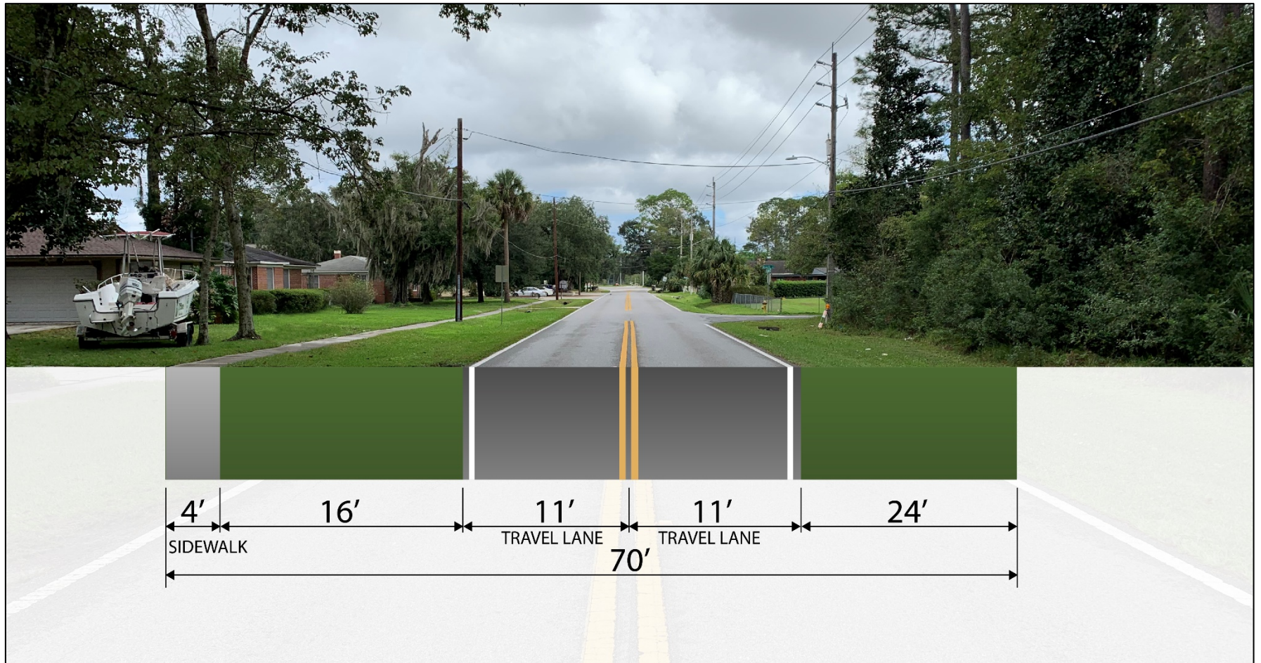
FIGURE 2-5 TYPICAL SECTION: SOUTH OF IBACH ROAD
