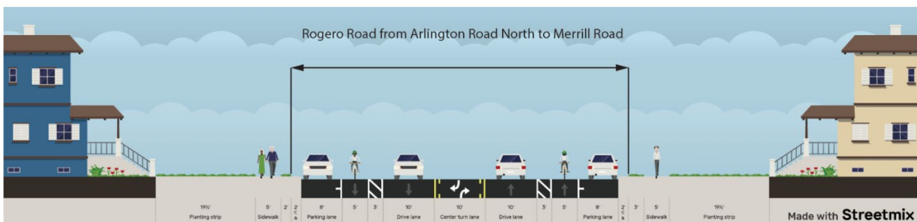
The lane repurposing concept includes buffered bike lanes and a two-way left turn lane. (Image: City of Jacksonville Planning and Development Department)
