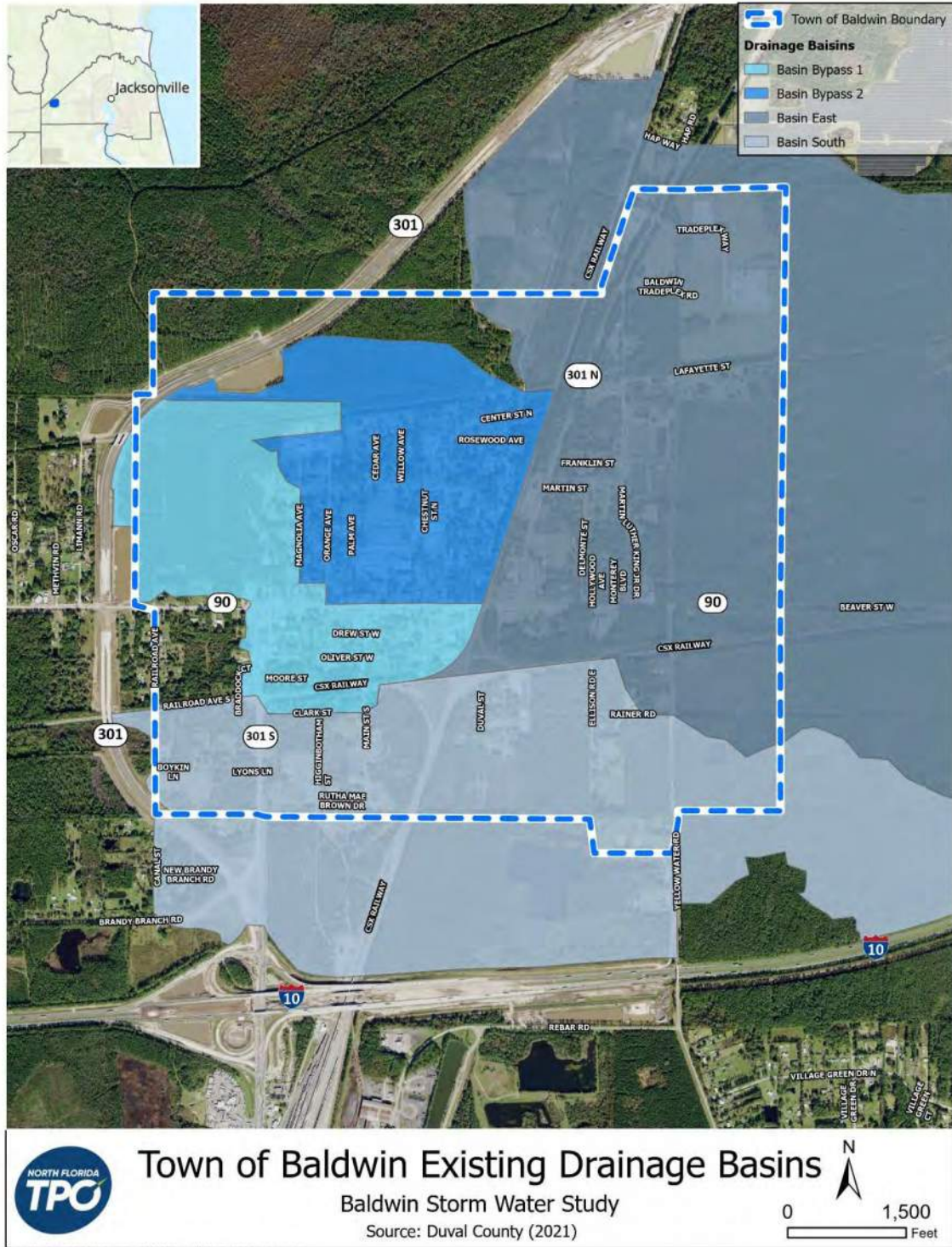
Figure 3. Existing Drainage Basins
